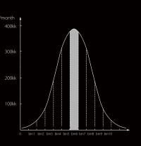
Monthly output of this model is greater than 400K. Lamps are selected from the same bin and batch to ensure consistency of brightness and color.
